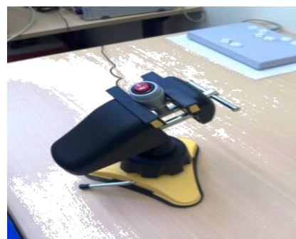
Figure 4-1: Vise Grip with MLA92 push-button attached. The push-button produced auditory feedback when fully depressed.
