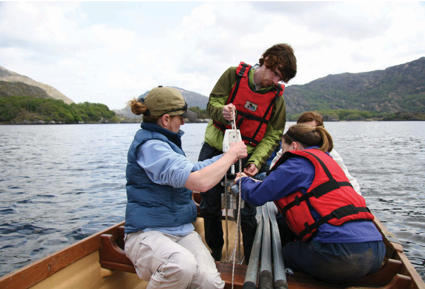
Figure 3.10 Collecting a short (< 50 cm) sediment core Upper Lake, Killarney.
